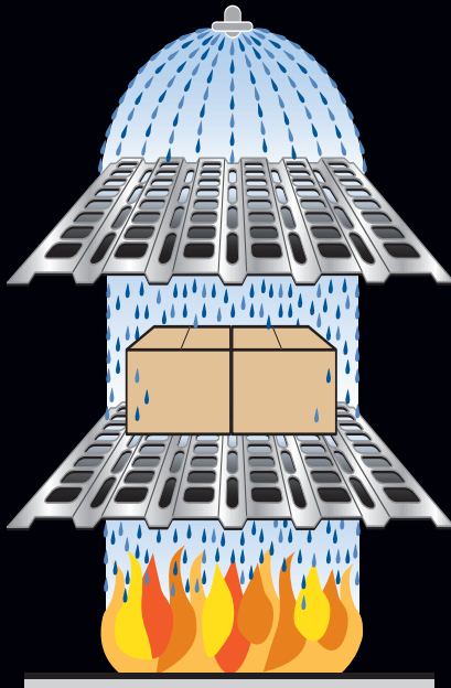
Punch Deck's open surface area allows sprinkler water through to lower levels.
